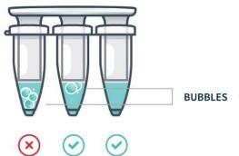
**Note:** Bubbles may remain at the top of a tube. This is acceptable. Bubbles at the bottom of the tube, however, are not acceptable.
