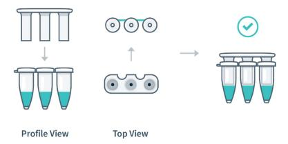
Hold the strip firmly between your fingers and use one finger to secure the void filling cap inside of the strip. Then, with a gentle whipping motion of the wrist, slowly flick the tubes a few times to ensure bubbles are removed from the bottom of each tube.
