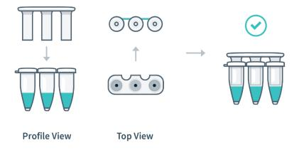
Hold the strip firmly between your fingers and use one finger to secure the void filling cap inside of the strip. Then, with a gentle whipping motion of the wrist, slowly flick the tubes a few times to ensure bubbles are removed from the bottom of each tube.
