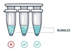
**Note:** Bubbles may remain at the top of a tube. This is acceptable. Bubbles at the bottom of the tube, however, are not acceptable.
